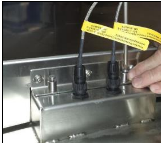
Figure 10 - Phillips Head Screws to Remove
