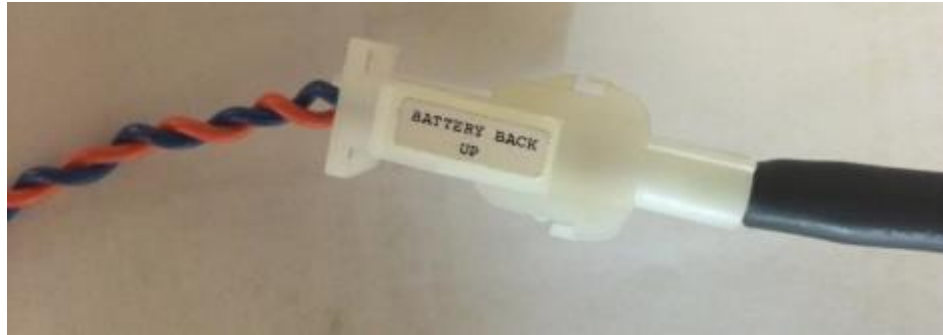
Figure 8 - Battery Backup Connector. [Black – From the Battery Backup. Dark Blue/Orange – From the TEC 3000 Wiring Harness]
