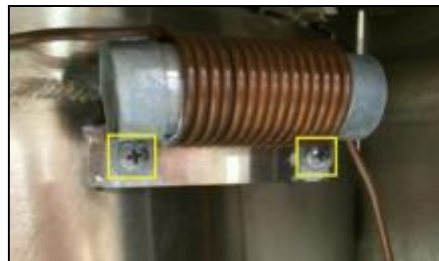
Figure 7 - Purge Coil Screws
