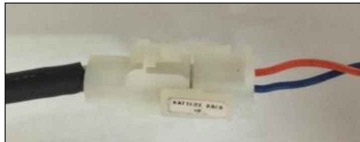
Figure 15 - Battery Backup Connector. [Black – From the Battery Backup. Dark Blue/Orange – From the TEC 3000 Wiring Harness]
