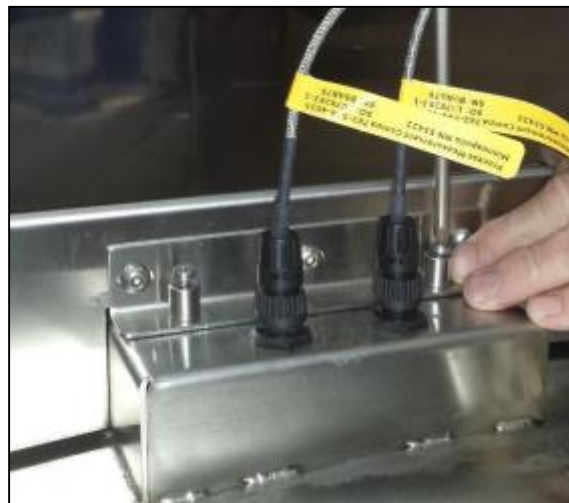
Figure 17 - Phillips Head Screws to Remove
