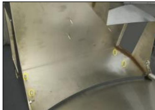
Figure 15 - Location to mount the battery backup
